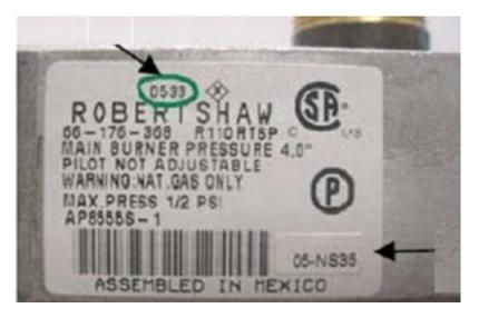
Unaffected valves on GSW and John Wood water heaters can be identified by a green line through the date code and a label that reads, "05-NS35." (See picture below.)
